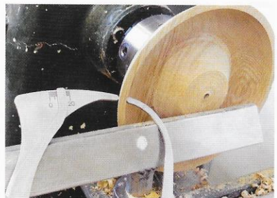
Hope callipers in use, the measuring scale shows exactly how much wood you have left
