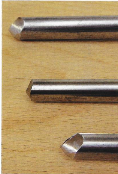
Different grind profiles of bowl gouges. The top and bottom are my personal preference of grind on different sized bowl gouges, the centre is a 'standard' grind
