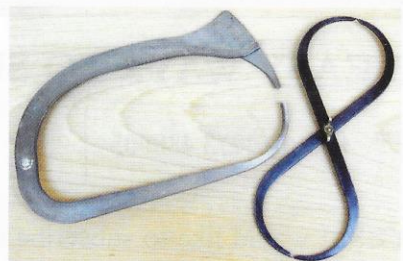
Traditional hour glass calliper – right – and the modern Hope calliper – left – which look strange but are the best type I have found for bowl work
