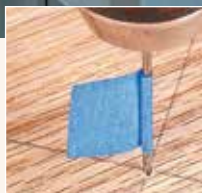
▲ Straight Cut First. After drilling a pivot hole (inset), place the workpiece on the jig. As you make the cut, hold the workpiece straight until the jig stops.
