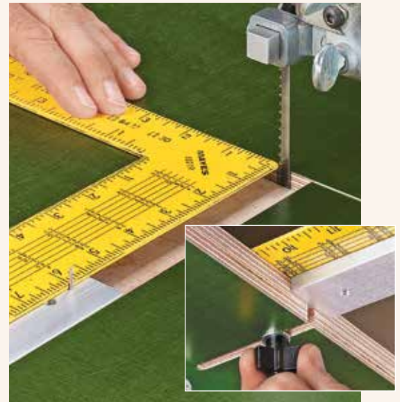
▲ Setting the Radius. To set the radius, loosen or remove the adjustment knob and slide the bar so the pivot pin is located at the desired radius and tighten the knob.
