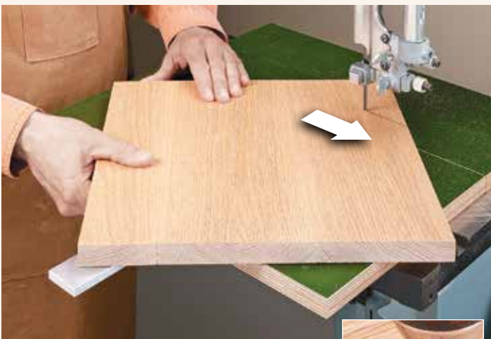
▲ Straight Cut First. After drilling a pivot hole (inset), place the workpiece on the jig. As you make the cut, hold the workpiece straight until the jig stops.
