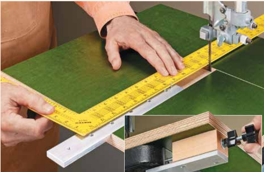
▲ Aligning the Center Pin. Use a framing square to align the pivot pin with the front edge of the blade. After adjusting the stop underneath so that the threaded rod contacts the table, lock it in place (inset photo).
