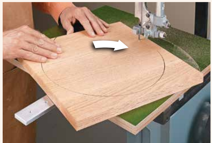
▲ Perfect Circles. Once the stop contacts the band saw table, you can start rotating the workpiece into the blade in a clockwise direction. The key to a smooth edge is to maintain a consistent feed rate throughout the cut.
