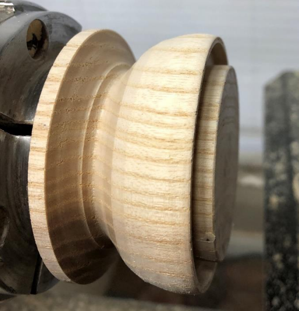
Begin shaping top of lid
