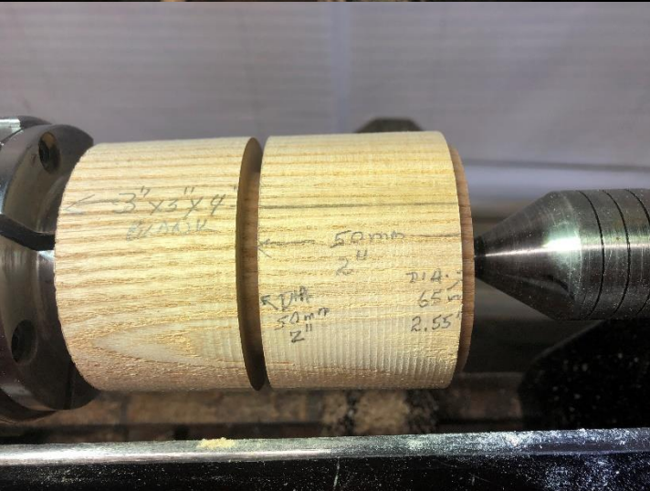
Base: Parted top and bottom diameters
