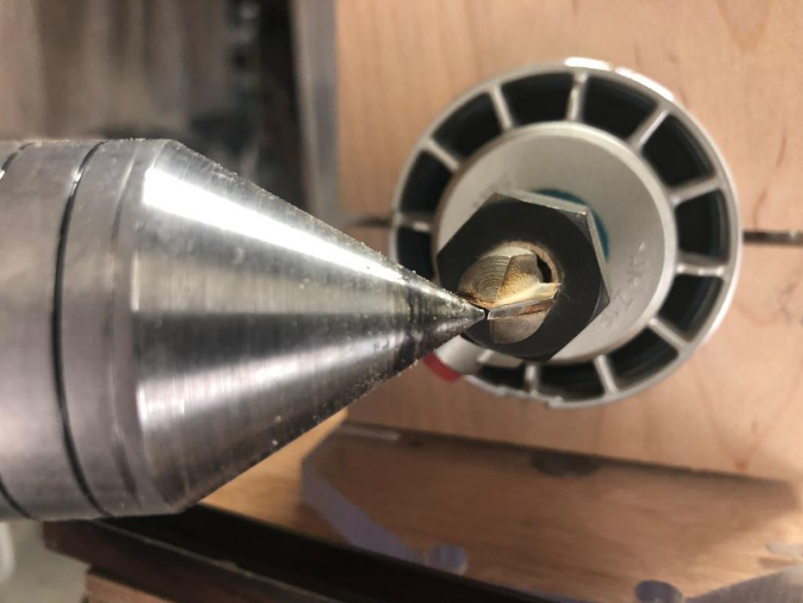
Align router bit to lathe centerline
