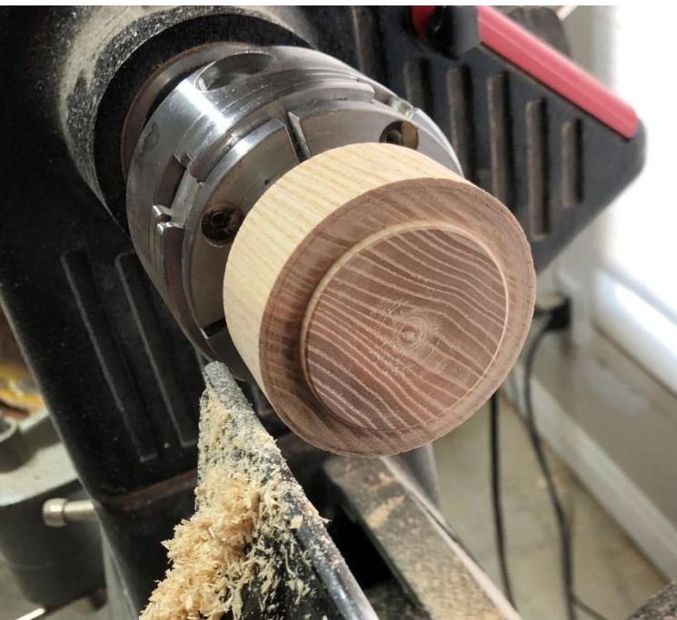
Measure base OD and cut tenon: ~ 53mm
