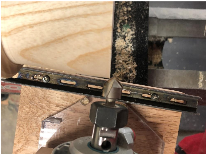
Align platform to match taper of cupcake base
