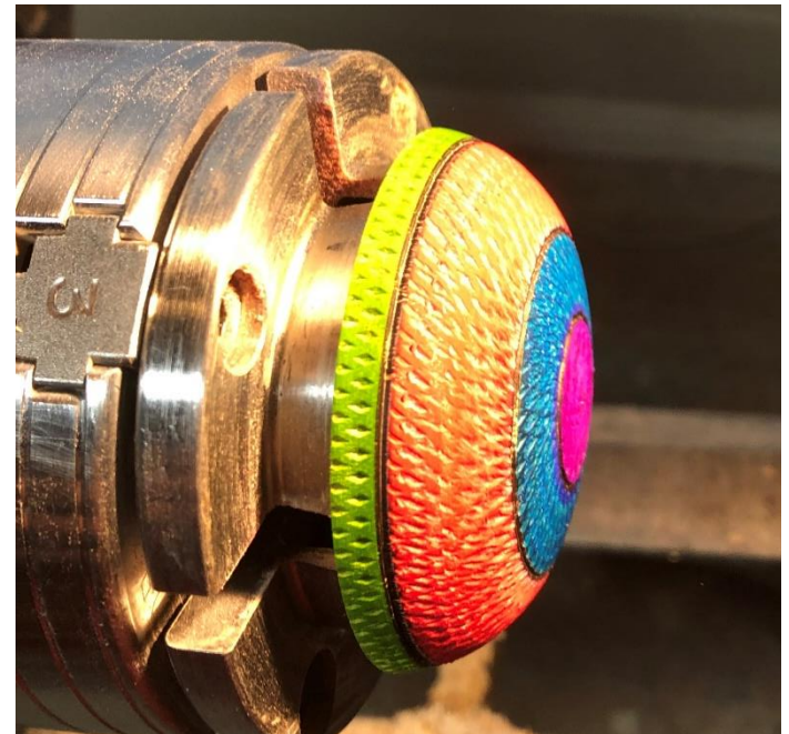
Knurl colored sections of lid at various angles
