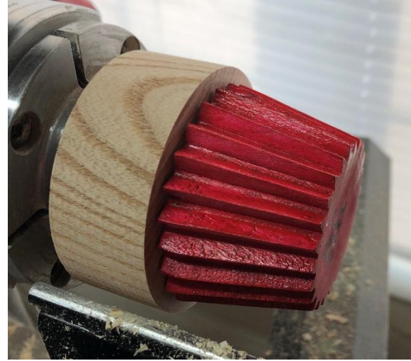
Use cupcake base to size tenon and mark OD of flutes on lid
