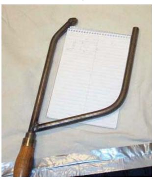
Note the size of this one is about 8 in wide and 10 inches long made with 5/8 inch stock, the pad is a standard steno pad, also note that it is rotated about the vertical axis in this photo. The cutter should be on the right.
