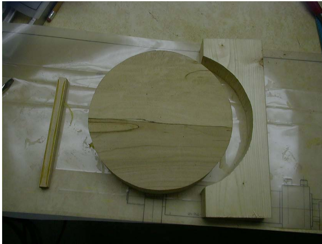
Preparing the maple for routing the groove
