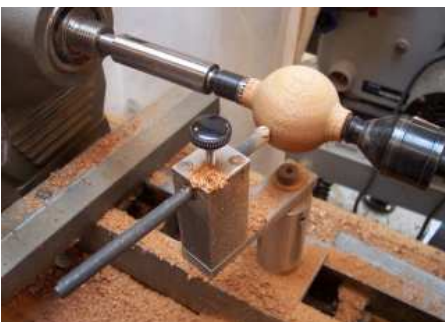
Figure 7. Sphere being cut with a Hunter 3/8" unhandled tool.
