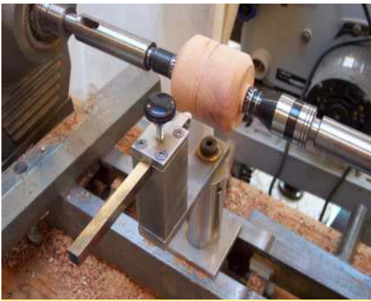
Figure 2. Starting the alignment of the jig so that the point of rotation (at the top of the shaft) is centered on the sphere blank. You can get approximate by setting the jig as shown here.
