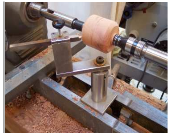
Figure 3. Swinging the jig to the left and set the cutter to just touch the corner of the sphere blank. The blank should be as wide as it is in diameter with a little extra toward the center for the drive and tail centers.
