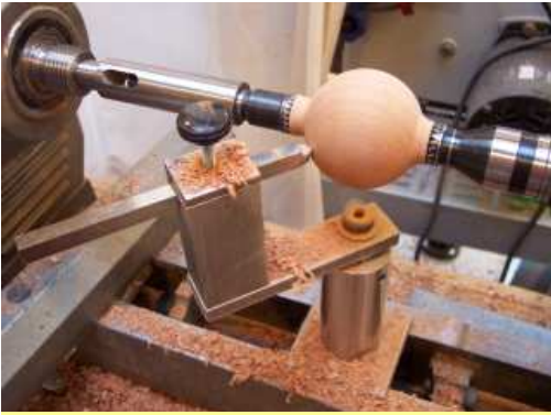
Figure 5. The sphere is now completed. The center line has just disappeared from the sphere.
