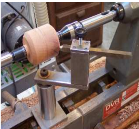
Figure 4. Jig swung to the right to check alignment.
