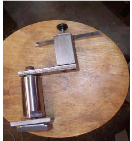
Figure 1. The Fred Lindsay Sphere Cutting Jig pictured here is designed to fit onto my Nova DVR lathe with a 16 inch swing.
