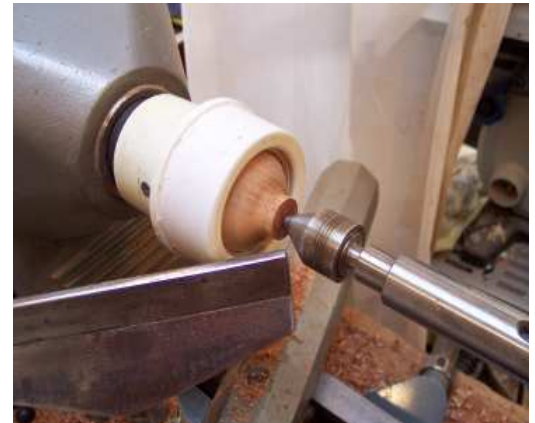
Figure 6. The sphere set up in a ball chuck to turn away the tenon.
