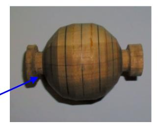
Part in a bit at each end of the sphere. Mark the centers between the 3 lines on the surface of the sphere and the corners where flats meet. These are orange lines on the right above. Then cut the corners off establishing flats between these lines. The centers of these flats will be on the surface of the sphere. Note: the photo on the left has the cross section of an 8-sided figure and the photo on the right has the cross section of a 16 sided figure.
