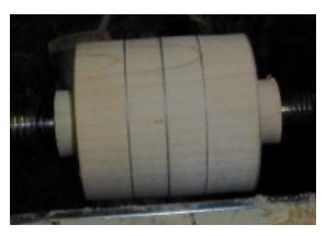
Part in on each end of the cylinder to create a tenon that is .41 of the desired diameter. Mark the two lines on the cylinder .41D apart centered about the centerline.
