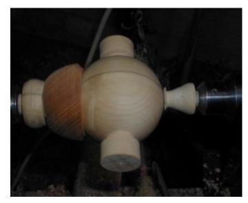
Using a cup of wood mounted at the headstock and a wooden pin over the live center press the ball into the cup. You can now turn off the stubs using light cuts with a bowl gouge cutting from the centers at each side up toward the middle of the tenon. As the ball rotates you see the outline of the sphere. Once you get close to sphere with cutting switch to scraping.
