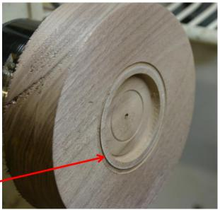
• Use a flat scraper or a parting tool to create an indentation deep enough for the chuck jaws when the wood is reversed.
