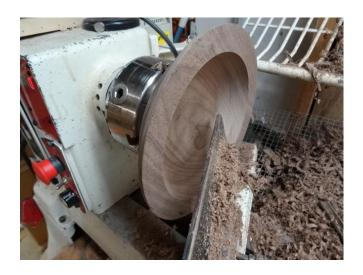
• Whichever method you use, keep checking the depth of the bowl with a depth gauge.
