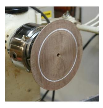
• Use a parting tool to start the hollowing process. Cut **parallel** to the outside of the bowl.
