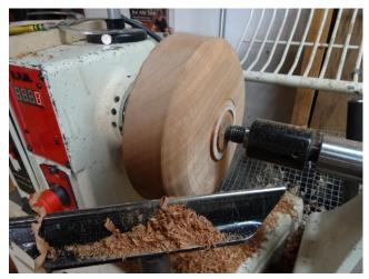
• Shape the bowl profile by eye or by using a template.
