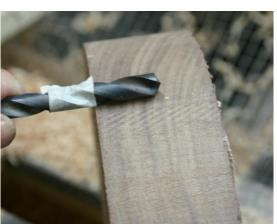
**Warning**: When measuring the size of hole to drill, measure the inner shaft –not the threads on the screw chuck.
