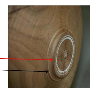
Whether using a tenon or a recess, make sure to leave a <u>flat</u> area that will rest against the jaws.
