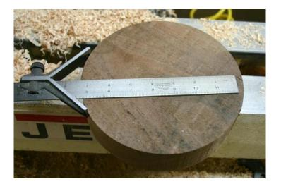
• Double-check with a compass and mark with a scratch awl.
