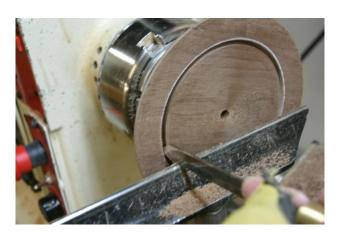
Starting a cut with a bowl gouge can be difficult for a beginner. Make two or three cuts with the parting tool.
