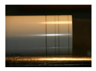
Use a parting tool to cut recesses that will fit the clamps. Make them uniform in depth.
