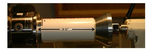
Mount the pipe in a chuck. True the right end. Reverse the pipe and true the other end.
