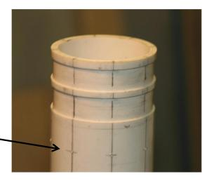
Using a  $\frac{1}{2}$ " brad point bit, drill four holes all the way through the pipe at each intersection.
