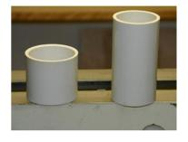
Mark a pencil line on the rim of the 4 ½" section of pipe.
