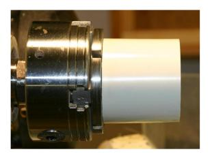
Seat the chuck into the coupling. Use a block of wood on the tailstock and slowly push the chuck into the coupling.
