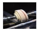
I drill a 1/8" hole in the center of the square so as to turn between centers. It's time to turn a tennon on the thickest piece of wood.
