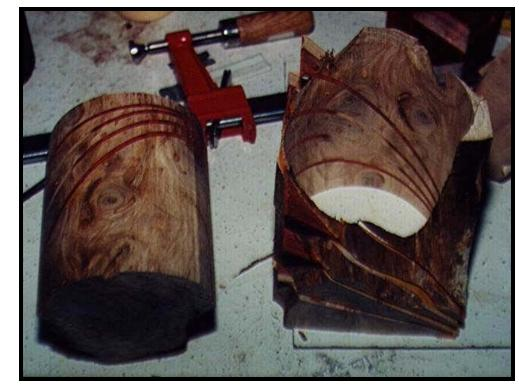
Layout and cut of "slug" on bandsaw
