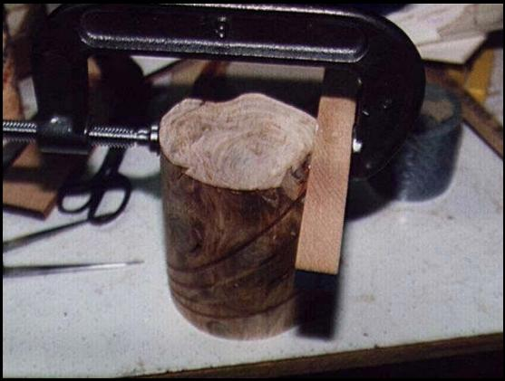
Preparation of slug for "V" groove on router table
