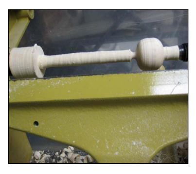
• Use the rougher gouge to reduced the handle to ½" diameter. Use the spindle gouge to shape the ball. Use the spear point scraper to finish the ball nose scraper to finish the neck to ¼" diameter.
