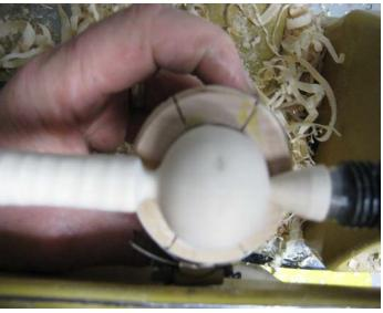
Use the fixture and the calipers to final size and roundness. Sand the ball.
