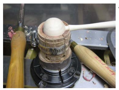
Orient the grain of the scoop either horizontally so that the annular ring shows at the bottom of the scoop or vertically so that the rings will show on either side of the scoop. The handle should swing in a flat arc. Tighten the hose clamp.
