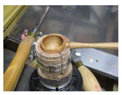
• Note how deep the fixture is. Add the side wall dimension to this and subtract 1/16 to get the depth of the bowl. Use a small bowl gouge and a ball nose scraper to finish the scoop. Push it out of the fixture with a piece of 3/8" dowel.
