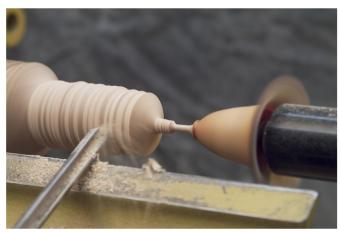
16 I continue with the same technique as before to remove wood and begin to thin the stem. Cutting downhill from left to right with bevel suported cuts (above and right)
