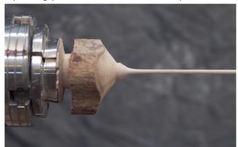
18 As you near the bottom section where you left the bark, form the base and add any detail you like at the base of the stem. Sand the base.
