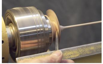
19 Start making slow parting cuts at an angle into the bottom of the base being careful not to catch the top edge of the parting tool on the rim of the base as it starts to get thin.
