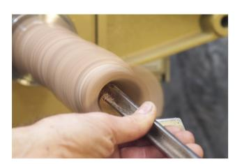
9 The interior of the goblet can be hollowed in several different ways. The generally accepted method for hollowing end-grain is back cutting from the center out toward the rim with either a spindle or bowl gouge. Here I am using a 5/8" fingernail grind bowl gouge. This cut is not a bevel supported cut but more of a scraping cut with the gouge flute rolled over toward the left side of the goblet interior.
