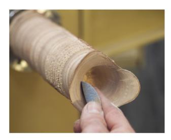
Now is a good time to.. **sharpen your gouge** and sand the interior of the goblet while there is still plenty of wood left on the outside for support.
