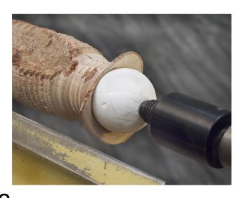
It is a good idea to support the goblet in some way when you continue shaping the outside and thining the stem. Here I am using a styrofoam ball available in different sizes at most craft stores. This goblet was very thin with several cracks around the rim so I chose a much smaller ball than shown above that would fit all the way inside the goblet. This put the pressure of the live center into the bottom of the goblet. The ball is not visible in the photos at left and below.
