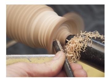
I will return to the inside and continue to shape the interior as much as possible with the tailstock in place. Keeping the tailstock in place reduces the vibration which helps give a better cut especially on longer goblets. For this I will use a 3/8" fingernail grind bowl gouge ground at about 40 degrees, this gives me a bit more clearance working arround the livecenter.
