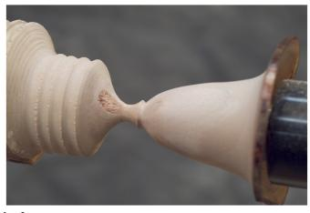
14 The soft pith area is visible in the waste wood portion and also in the bottom of the goblet. This will be turned away as we turn the stem but the area in the goblet will need to be delt with.
