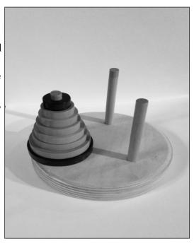
When I make this puzzle, I usually plan on making at least 4 of them. The reason is that i turn all eight diameters of the discs separately. This is so I end up with 8 cylinders with 8 diameters from 2" to about 3/4". Before I take a cylinder off of the lathe, I drill a 5/16" hole. I make the hole deep enough to make between 4 and 6 cuts on my chop saw.
