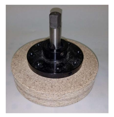
Clamp a metal faceplate over the predrilled hole in your wood faceplate and then run the tap into the wood. This will ensure that the tape goes in straight.
