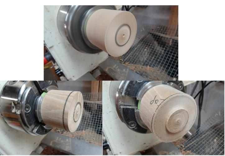
Form a tenon  $\frac{1}{2}$  deep at the bottom of the cap that will fit inside the **1** 3/8 hole drilled previously at the top of the **body** of the mill. The fit does not have to be snug, but not too loose.
