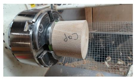
Remove the **body** from the lathe and mount the **cap**.
