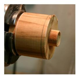
Turn the tenon to 1 1/16'' and fit it to the body.
