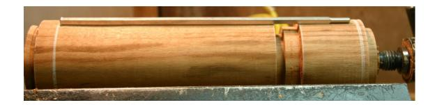
Mark  $\frac{1}{2}$ " from the bottom and lay the mill shaft on top and mark.
