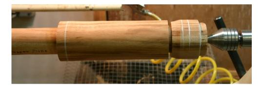
Mount the peppermill jam chuck and assemble the body as above.
