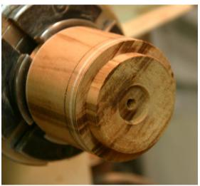
Drill a 7/8" hole for the shaft mechanism.
