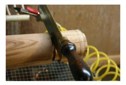
Saw off the top. Make sure to leave a tenon for the body.
