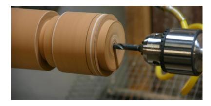
Drill a 9/32" hole through the top and into the main body.
