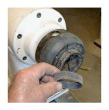
A piece of a small tire tube is cut and put over the jaws of the chuck to protect the inside of the bracelet.
