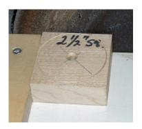
Using a disk sander remove the material up to the line.
