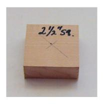
Start with a waste block the thickness of the bracelet you want to make. Mark the center as close as possible. I have marked the center off for illustration purposes. Drill a ¼ in hole and countersink this will hold the piece at center each time it is remounted.
