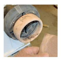
Shape the outside and inside edge, turn around and do the other edge. Sand until you're satisfied. I do not finish on the lathe.
