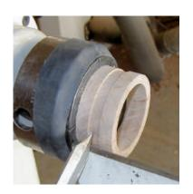
Remove the wood to the depth of the inlay with a standard parting tool.
