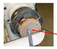
Use a narrow parting tool that has a modified tip.
