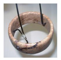
Put on one or two coats of sanding sealer and hand sand. With a 3 prong spring holder I spray 2 to 3 coats of lacquer.
