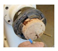
With a compass set to ½ the inside diameter draw a line to mark for the parting tool.
