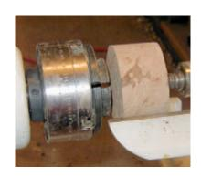
Mount the block to the lathe using the front of the chuck jaws as a jam chuck. True up the outside to the desired diameter.
