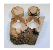
Cut the circles out on a band saw.
