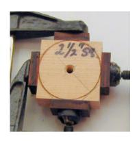
1st glue up. Use ¼ in. thick material, this is Rose Wood. Make each segment long enough to cover when the corners are cut off. I use Epoxy in most of my lay-ups. Clean all surfaces with Acetone especially on exotic woods.
