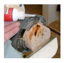
Fill any cracks or voids with CA glue.
