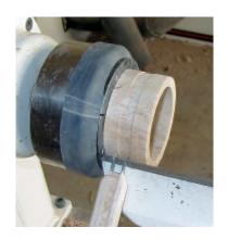
Use skew chisel to cut the fibers where the inlay will be placed. I made a tool with two blades. Made from saber saw blades and pointed, then sharpened on the inside. This will cut the same each time.
