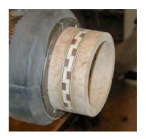
Remove tape and mount on lathe. Shape and sand.
