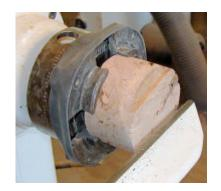
True up the face of the block to the desired width, marking the center with an indentation.
